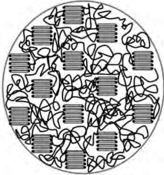
Figure 9.2 Schematic representation of the structural model of PVA/PEG double-network hydrogel.
