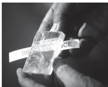
Fig. 2.7 The birefringence of calcite (Iceland spar).
