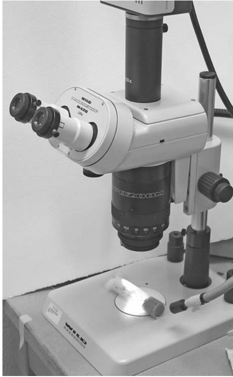
Fig. 4.16. A research grade stereomicroscope. Note the light source is from the side, which can give a shadow effect to the specimen – in this example a vial of flies. The large objective lens above the specimen can be rotated to zoom the image.
