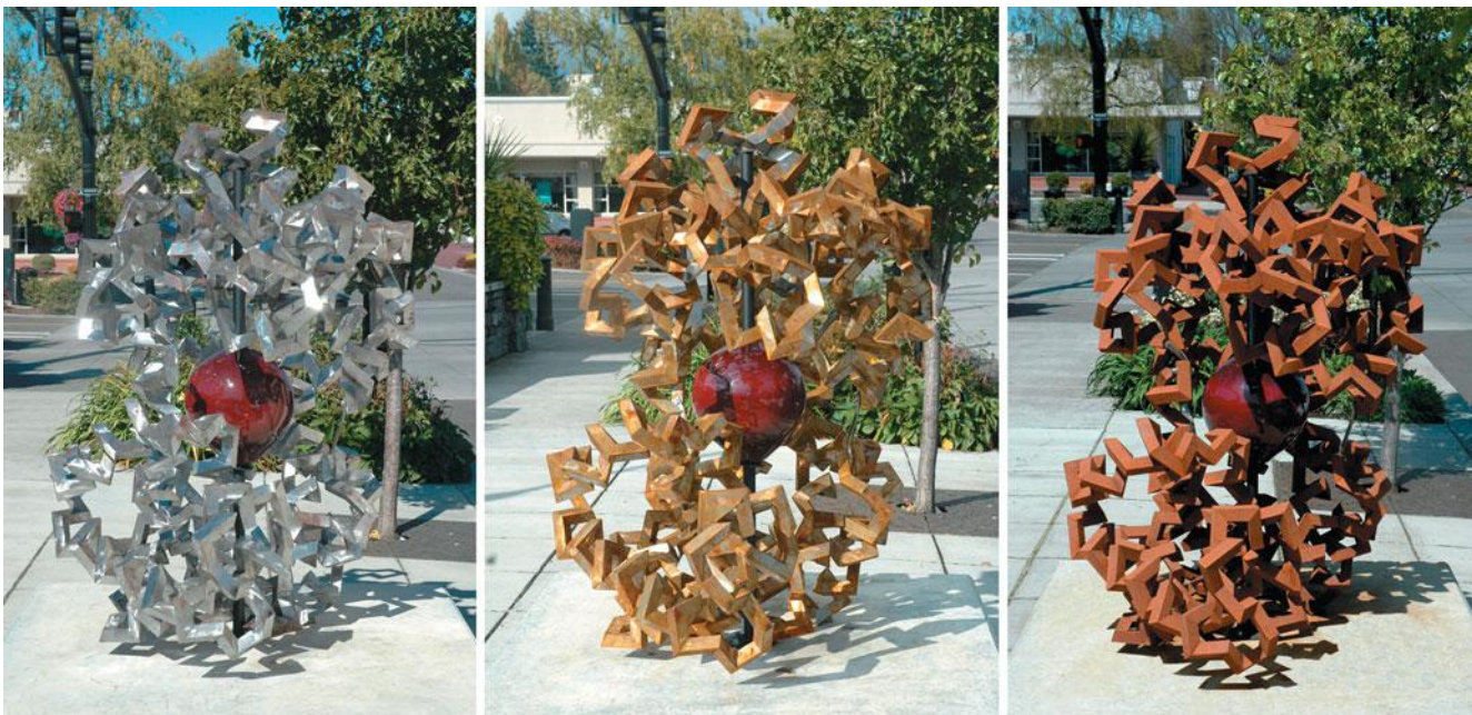
▲ Julian Voss-Andreae created a sculpture called “Heart of Steel (Hemoglobin)” in 2005 in the City of Lake Oswego, Oregon. The sculpture is a depiction of a hemoglobin molecule with a bound oxygen atom. The original sculpture was shiny steel (left). After 10 days (middle) it had started to rust as the iron in the steel reacted with oxygen in the atmosphere. After several months (right) the sculpture was completely rust colored.
