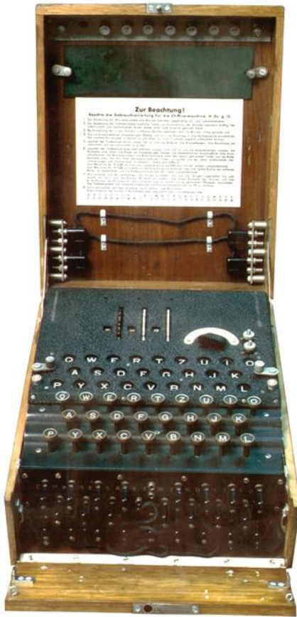
▲ The enigma cryptography machine used by German armed forces during the Second World War. This mechanical typewriter permitted the user to adjust its three large dials to encrypt outgoing messages before being sent by telegraph. The recipients could decode the message by setting the dials on their enigma machine to match. This type of encryption is extremely difficult to decipher, but when Allied forces were able to capture an intact enigma machine they could listen in on all their enemy's transmissions.
