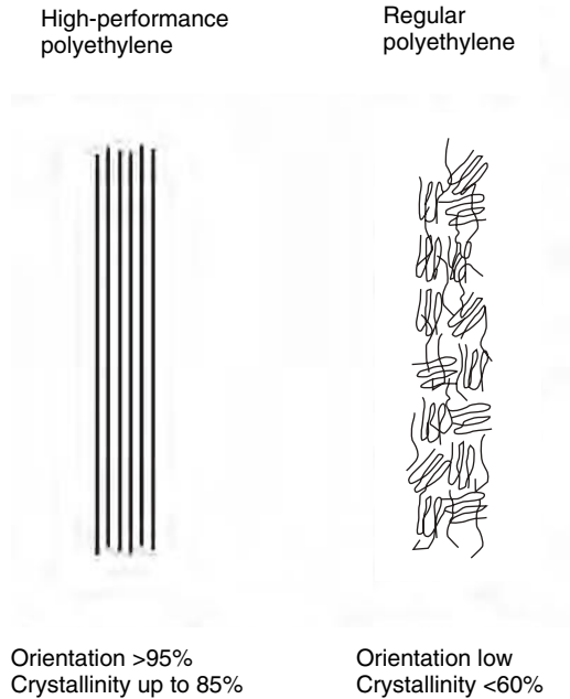
3.1 Macromolecular orientation of HPPE and normal PE.
