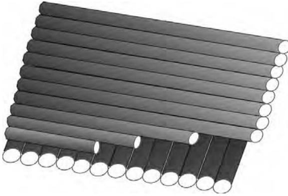
3.12 Construction of Dyneema UD and Spectra Shield .
