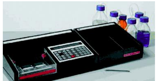
Figure 9.25 An automated electrophoresis system. The left-hand compartment performs electrophoretic separation of proteins on thin, uniformly made, gels whilst the second compartment performs the staining reaction to visualize protein components. The gels are run horizontally. (Reproduced courtesy of Amersham Biosciences)
