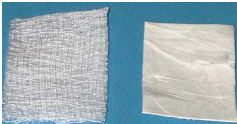
Figure 3. Photograph of a cotton gauze (left) and an electrospun bovine fibrinogen mat (right) produced from 0.167 g/ml fibrinogen in HFP/MEM that is approximately 6 x 6 cm with a thickness of 0.7 mm (dry mass is approximately 0.08 grams) for potential use as a tissue engineering scaffold or wound dressing.
