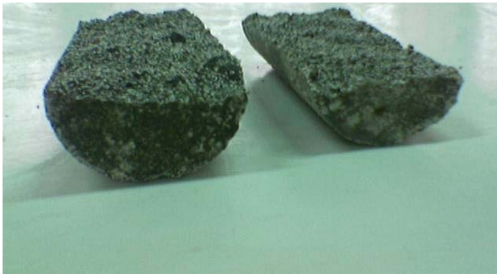
Figure 21. The failure mode in EPS glasscrete.
