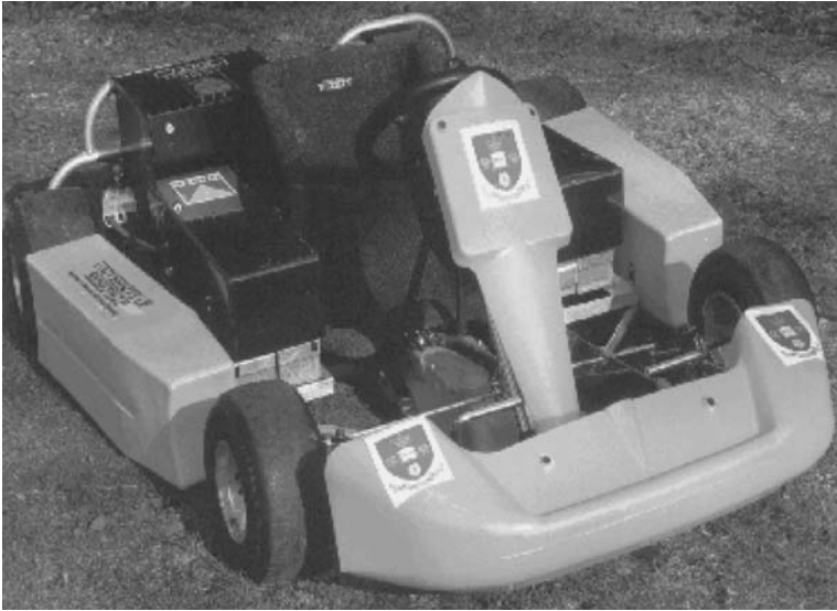
Figure 4.28 The all-electric go-kart. Photo courtesy of Professor D. Howe, University of Sheffield
