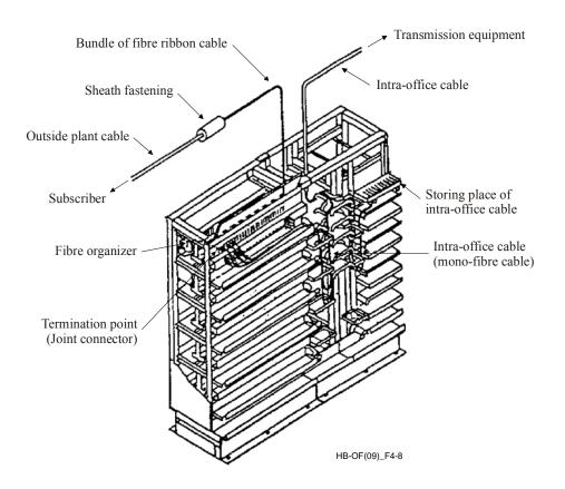
Figure 4-8 – Optical fibre distribution frame (without jumpers)
