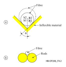
Figure 4-2 – V-groove or two-cylinder alignment
