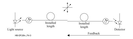
Figure 4-3 – Example of active core alignment
