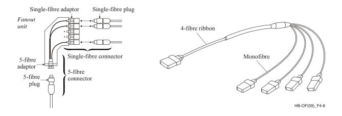
**Figure 4-6 – Fanout connectors**
