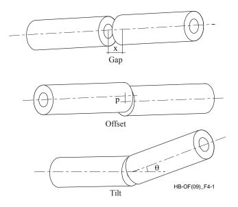
Figure 4-1 – Fibre misalignment
