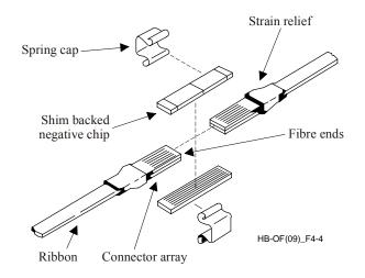
Figure 4-4 – Multiple fibre mechanical splice
