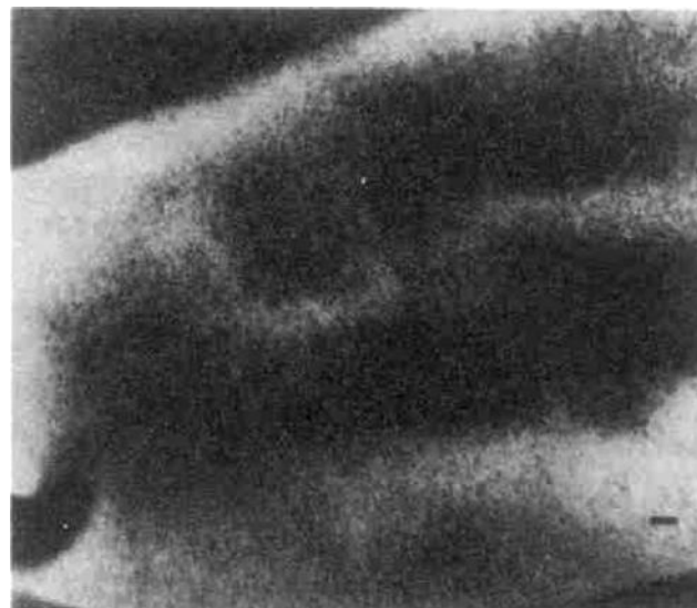
FIGURE 32.1. Transmission electron micrograph for PDMS filled with silica using basic catalysts. From [2] 1988 © John Wiley and Sons.
