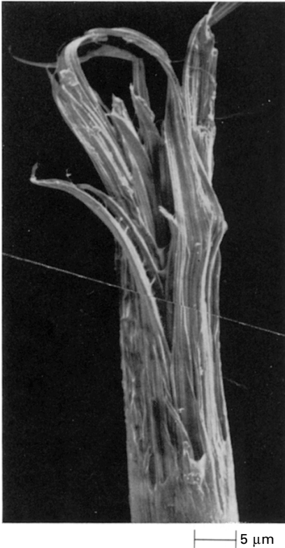
19.17 Fibrillar break of wet mercerised cotton.
