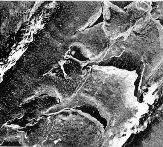
25.16 Acetate fibre abraded by passing over a ceramic guide at 300 m/min. Damage is due to fibre sticking to a guide and then breaking away [4].
