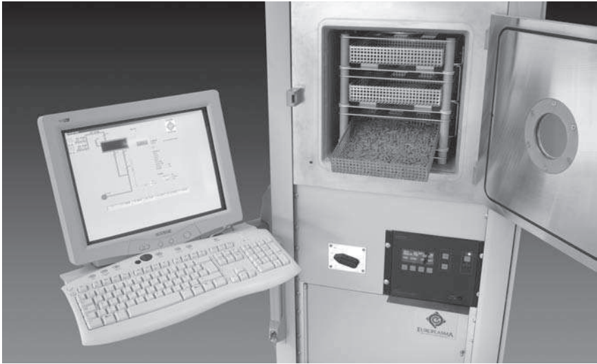
3.2 Vacuum plasma chamber with a classical loading system consisting of a set of trays.
