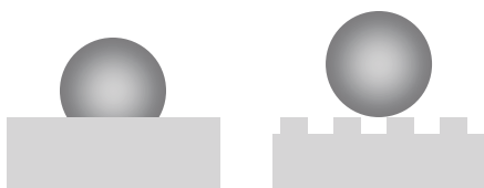
7.1 Super hydrophobicity resulting from surface roughening of a hydrophobic surface.
