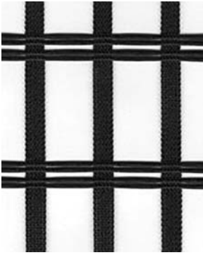
18.11 Knitted high tenacity polyester geogrids with UV stabilized saturation coating [31].
