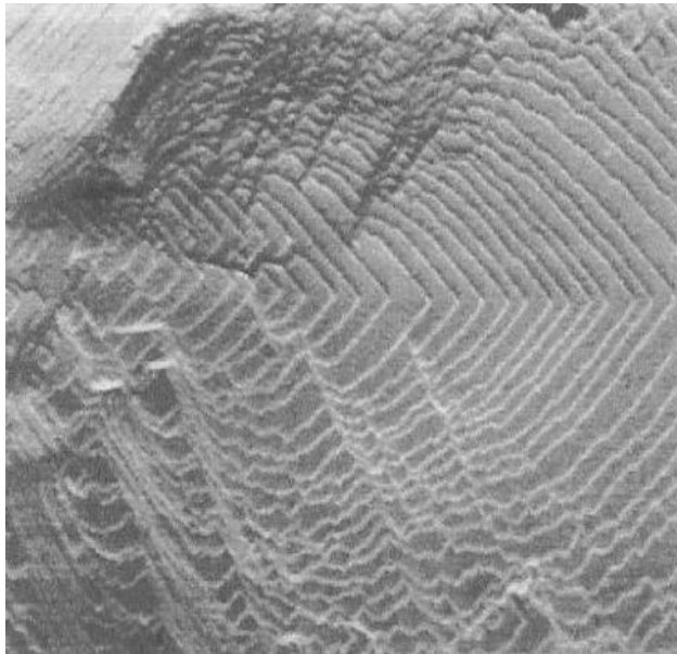
Figure 2.18 Atomic force microscopy images of an area 3.5\ \mu\text{m} \times 3.5\ \mu\text{m} of poisoned growth of calcite. 46
