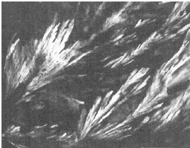
Figure 5.13 Thin film of polypropylene, part of spherulite crossed polars. 31
