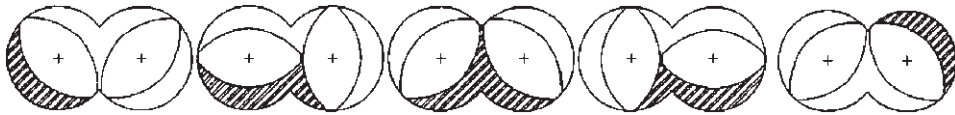
Fig. 10.11 Snapshots of the repetitive expansion/contraction of each of the cross-sectional area “pockets” between a pair of kneading disks and the barrel of fully intermeshing, co-rotating extruders. The evolution of the expansion/contraction is followed for one of the three “pockets,” the one shaded, A_s(t) .
