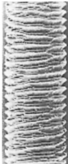
Fig. 12.17 Scanning electron micrograph of HDPE extruded at a shear rate slightly lower than the oscillation region, showing "sharkskin." [Reprinted by permission from N. Bergem, "Visualization Studies of Polymer Melt Flow Anomalies in Extruders," Proceedings of the Seventh International Congress on Rheology , Gothenberg, Sweden, 1976, p. 50.]
