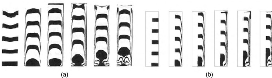
Fig. 13.28 Deformation of ABS at different piston displacements: 0, 11, 22, 33, 44, and 55 mm. (a) Experimental. (b) Calculated using a Bingham fluid model ( T = 230^{\circ}\text{C} ). [Reprinted by permission from E. Vos, H. E. H. Meijer, and G. W. M. Peters, "Multilayer Injection Molding," Int. Polym. Process. , 6 , 42 (1991).]
