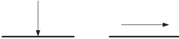
Fig. 6.1 The two basic machine elements: a plane moving normal to its plane and a plane moving parallel to its plane.
