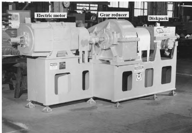
Fig. E9.7b Photograph of a 350-mm-diameter co-rotating disk Diskpack 16 compounder manufactured by the Farrel Corporation with a tested production capacity of 3000 lb/h. [Courtesy of Farrel Corporation, Ansonia, CT.]
