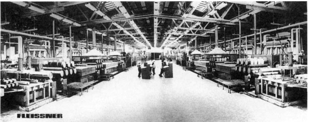
Figure 1.17 Two-stage fiber aftertreatment lines for approximately 200 tons/d capacity [43]
