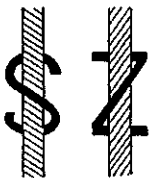
Figure 3.32 Definition of the twist direction (S respectively Z)
