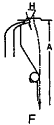
F) Slit quench chamber H < 0.05 \text{ m} Q \geq 40 G v \geq 10 \text{ m/s} For PET and PP compact staple fiber spinning
