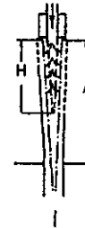
I) Radial quench chamber As H, but with air inlet from above, through core of spinneret
