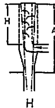
H) Radial quench chamber (outside \rightarrow inside) H \leq 1.2 \text{ m} Q \approx 16 G v < 1.0 \text{ m/s} weakly turbulent
