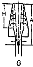
G) Radial quench chamber (inside \rightarrow outside) H \leq 1.2 \text{ m} v \approx 0.4 \dots 1.0 \text{ m/s} Q \approx 8 \text{ (for PET)} \dots 25 \text{ (for PA)} \times G \text{ [kg/h]} Preferred for staple tow (in vertical spinning) Number of spinneret holes > 2000
