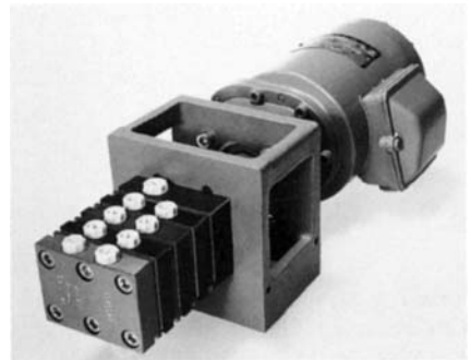
Figure 4.194 Spin finish pump assembly for many yarn ends, fitted with gear tooth pumps as per Figure 4.114 and a small, geared reluctance motor of 40...60 W to give 8...60 rev/min [24, 87, 106, 107]
