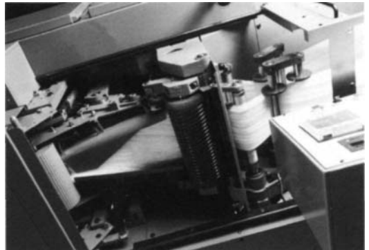
Fig. 5.71 Schematic and photograph of the cutting zone of a Schlumberger Converter [166]
