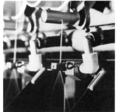
Figure 7.22 Intermingling jet [33] incorporating a noise-reduction principle (ca. 80 dB at 6 bar), air consumption at different pressures and a photograph of it mounted on a drawtwister
