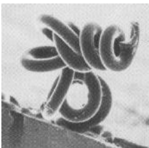
3.1 Monville , which was a nylon/elastomer bicomponent fibre, after rupture.
