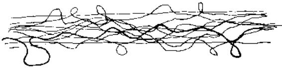
3.8 Schematic illustration of yarn structure. From Kollu (1985).
