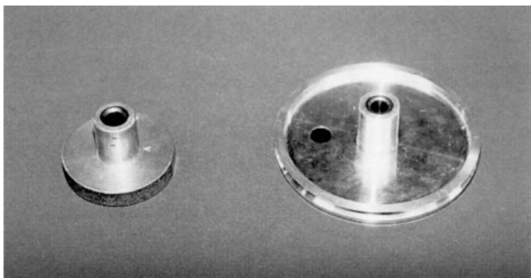
7.7 A Swiss pilling holder compared with a standard holder.
