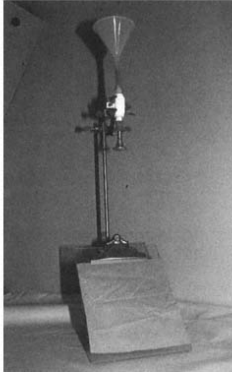
Figure 7 Spray impact tester used for testing in accordance with AATCC 42 and FTMS 191A,5222. (Courtesy of TRI/Environmental, Inc.)
