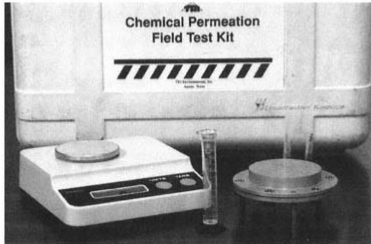
Figure 5 Permeation test cup and field test kit conforming to ASTM F1407, which may also be used for measuring barrier material chemical degradation resistance. (Courtesy of TRI/Environmental, Inc.)
