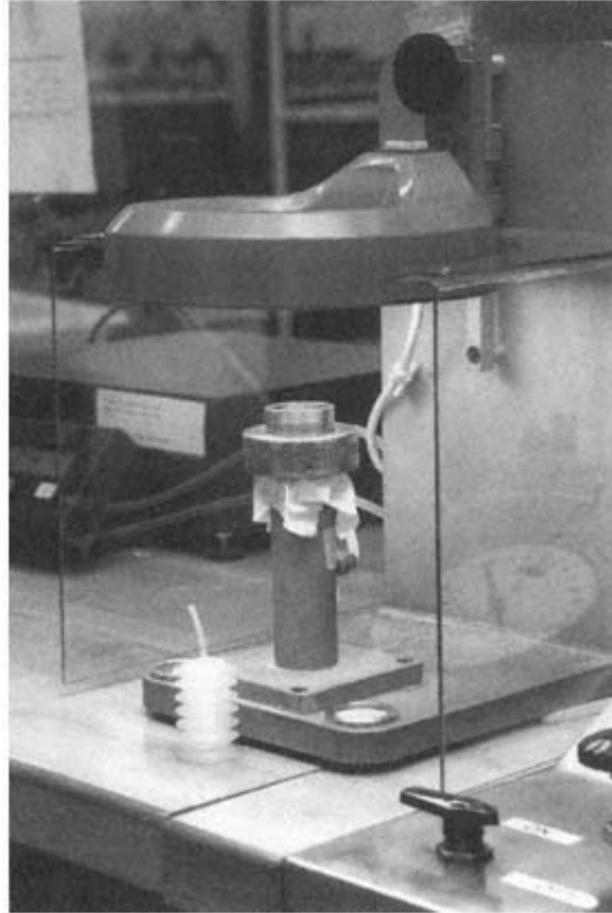
Figure 39 The maximum pore size of nonfibrous porous film reinforcements used in textiles can be approximated using ASTM F316-86 (Standard Test Methods for Pore Size Characteristics of Membrane Filters by Bubble Point and Mean Flow Pore Test).
