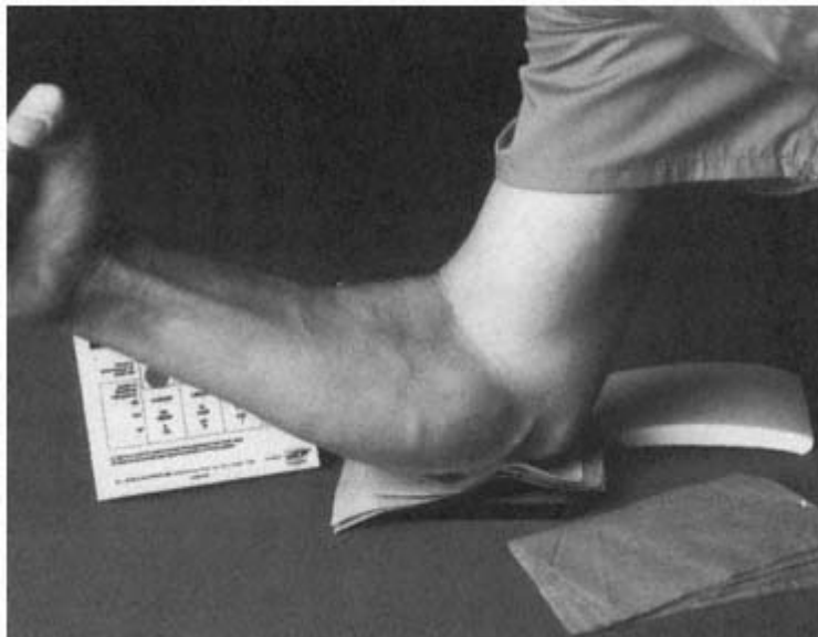
Figure 27 The GORE elbow lean test. Contact W. L. Gore & Associates, Inc., for details on how to order test kits [11].
