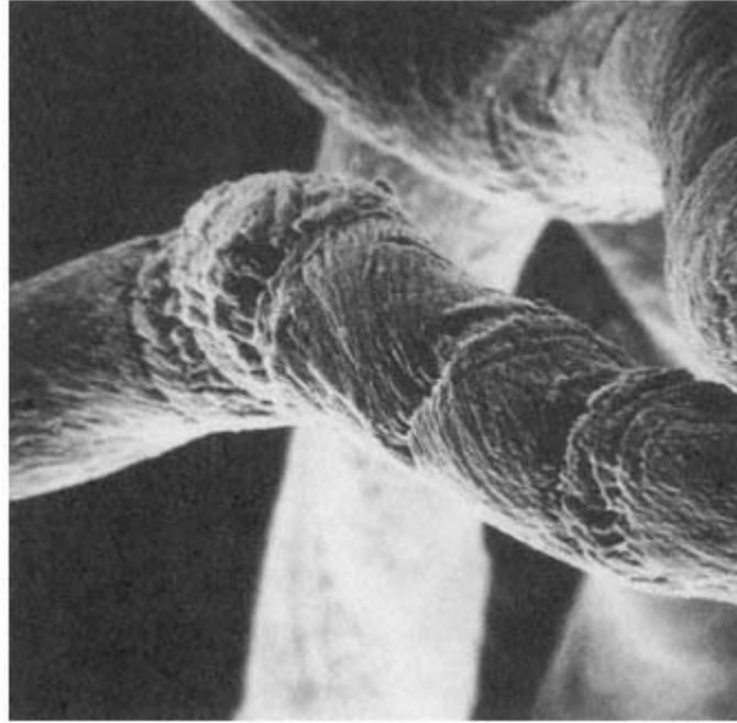
Figure 10 Fungus-damaged fiber after sodium hydroxide swelling.
