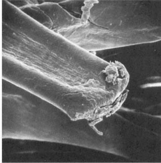
Figure 8 Blunt end of a broken, dry-abraded fiber.
