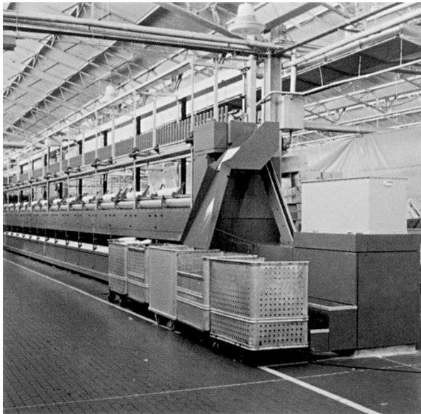
Fig. 93 Bobbin unloading and tube reloading
