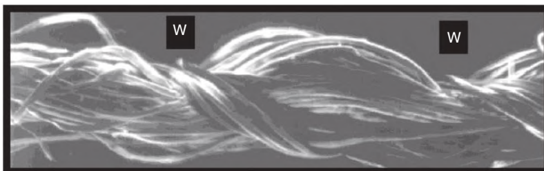
Fig. 10.6 Micrograph of an air-jet yarn
