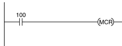
Figure 1.8 Master Control Relay
