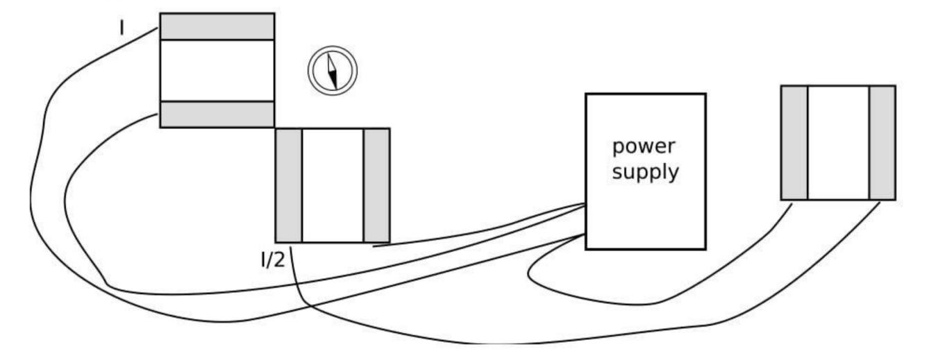
Try it. To cut the current to one of the solenoids in half, an easy and accurate method is simply to put the third solenoid in series with it, and put that third solenoid so far away that its magnetic field doesn't have any significant effect on the compass.
