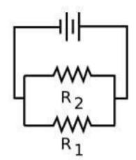
Insert your multimeter in the circuit to measure all three currents that you need in order to test the junction rule.
