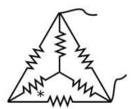
This is unfortunately a circuit that cannot be converted into parallel and series parts, and that's what makes this a hard problem! However, we can recognize that by symmetry, there is zero current in the resistor marked with an asterisk. Eliminating this one, we recognize the whole arrangement as a triple parallel circuit consisting of resistances R, R, and R. The resulting resistance is R.
