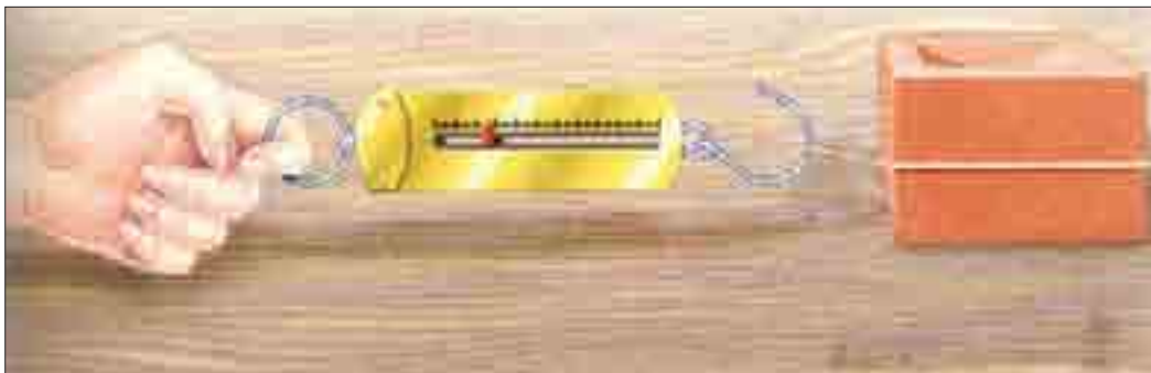
The pointer of this spring gauge shows the tension in the hook as the brick is pulled along.
