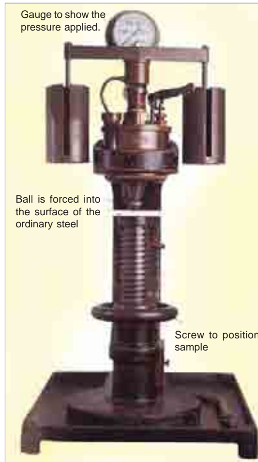
Brinell Tester : Hardness can be defined as the resistance of a metal to attempts to deform it. This machine invented by the Swedish metallurgist Johann August Brinell (1849-1925), measure hardness precisely.
