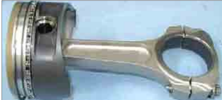
Piston rod is made of mild steel.
