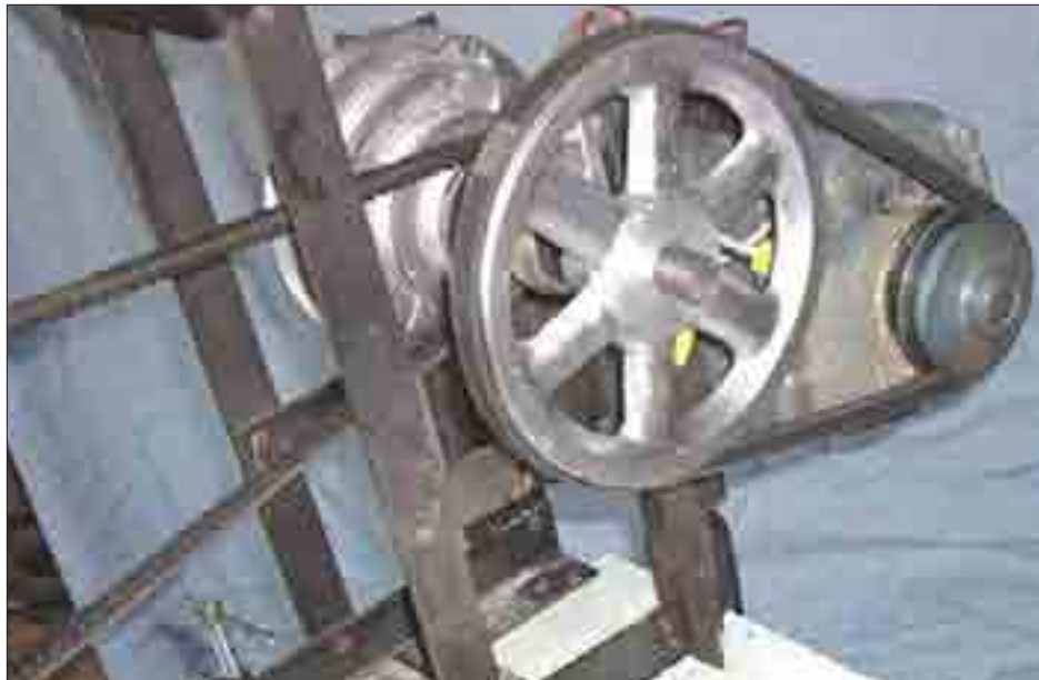
Belt drive on a lathe
