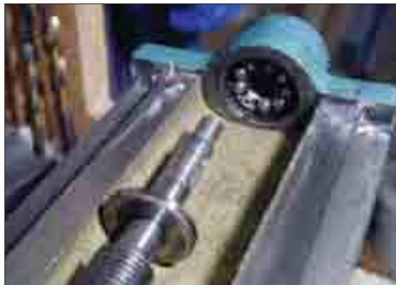
Lead screw supported by collar bearing.
