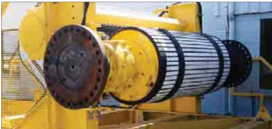
This massive shaft-like pulley drives the conveyor belt.
