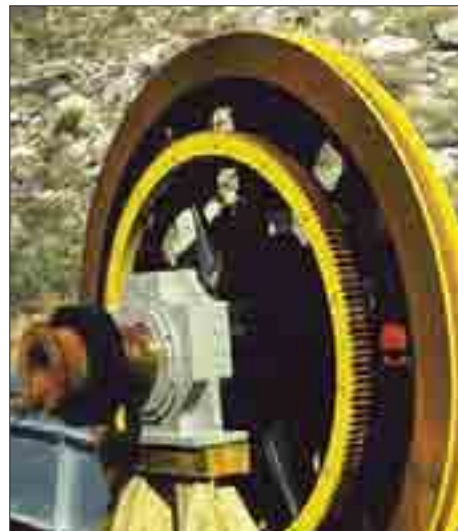
Wheel that winds the metal rope.
