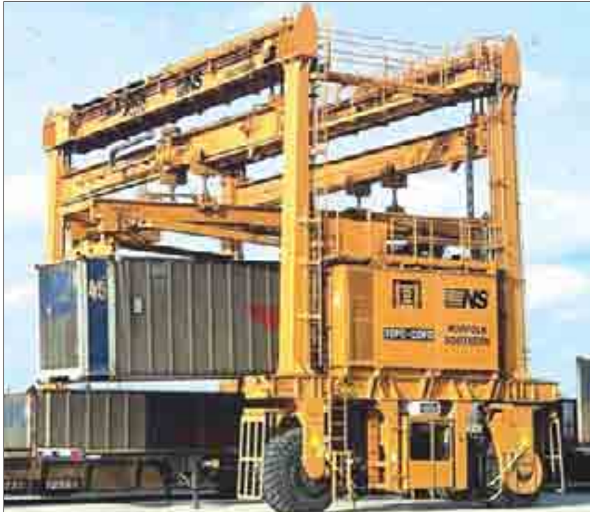
A heavy duty crane. Cranes use rope drives in addition to gear drives
