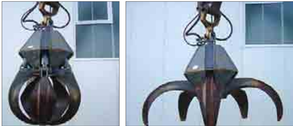
5-tine clamps of a material handler
