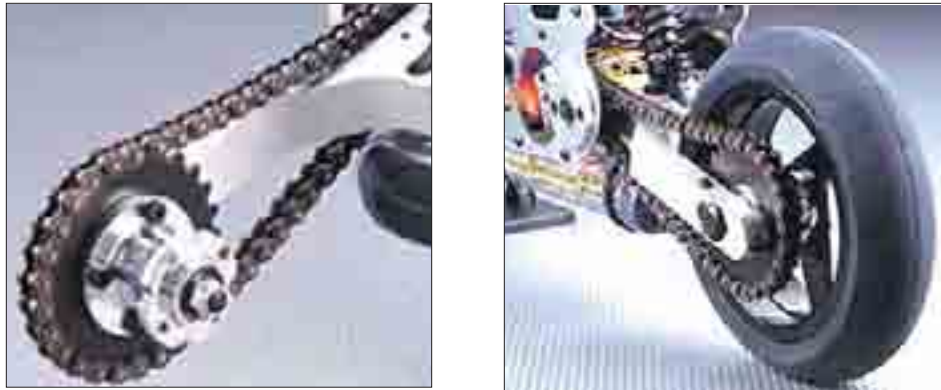
Rear wheel chain drive of a motorcycle
