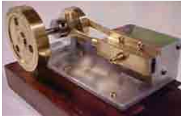
Flywheel stores energy when the supply is in excess, and releases energy when the supply is in deficit.
