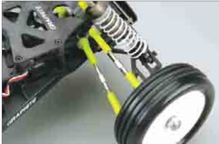
An automobile suspension and shock-absorber. The two links with green ends are turnbuckles.
