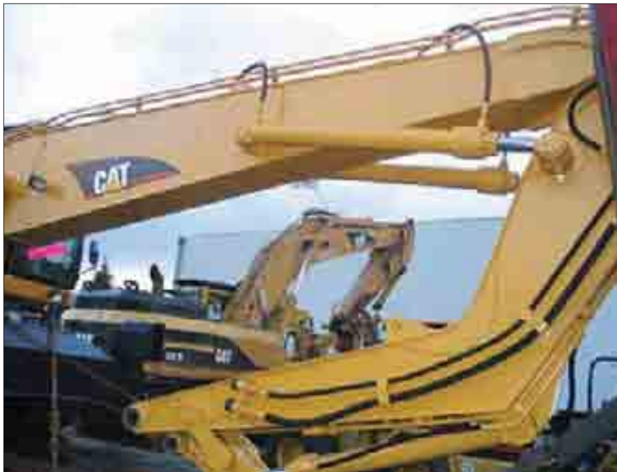
Arm of a material handler In addition to gears, hydraulic rams as shown above, play important role in transmitting force and energy.
