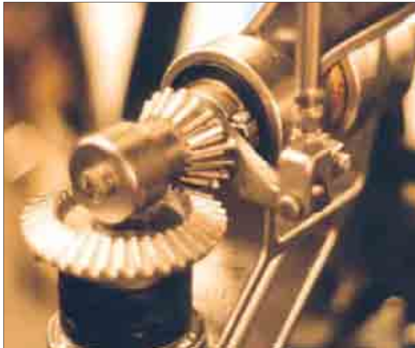
Fig. 30.1. Pitch surface for bevel gears.
