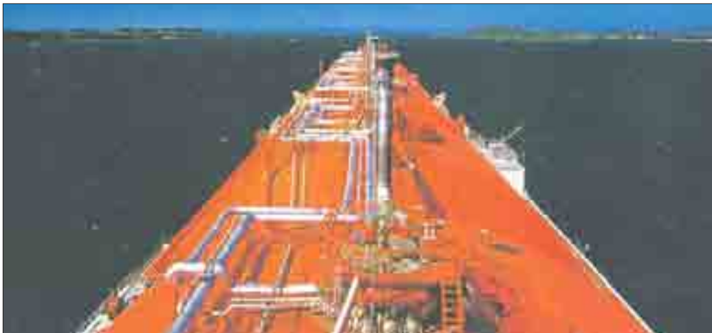
This view along the deck of a liquefied natural gas (LNG) carrier shows the tops of its large, insulated steel tanks. The tanks contain liquefied gas at -162^{\circ}\text{C} .
