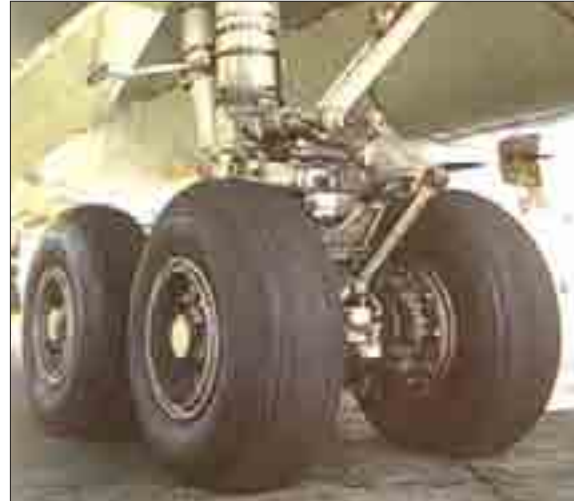
Main wheels on the undercarriage of an airliner. Air plane landing gears and wheels need to bear high stresses and shocks.
