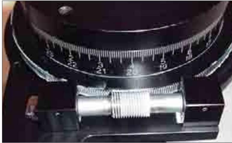
The worm in its place. One can also see the two cubic worm bearing blocks and the big gear.
