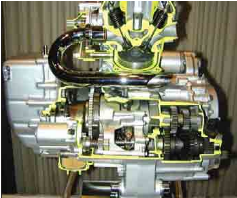
Water cooled 4-cycle diesel engine
