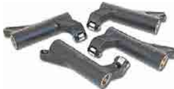
Roller followers in an engine rocker mechanism
