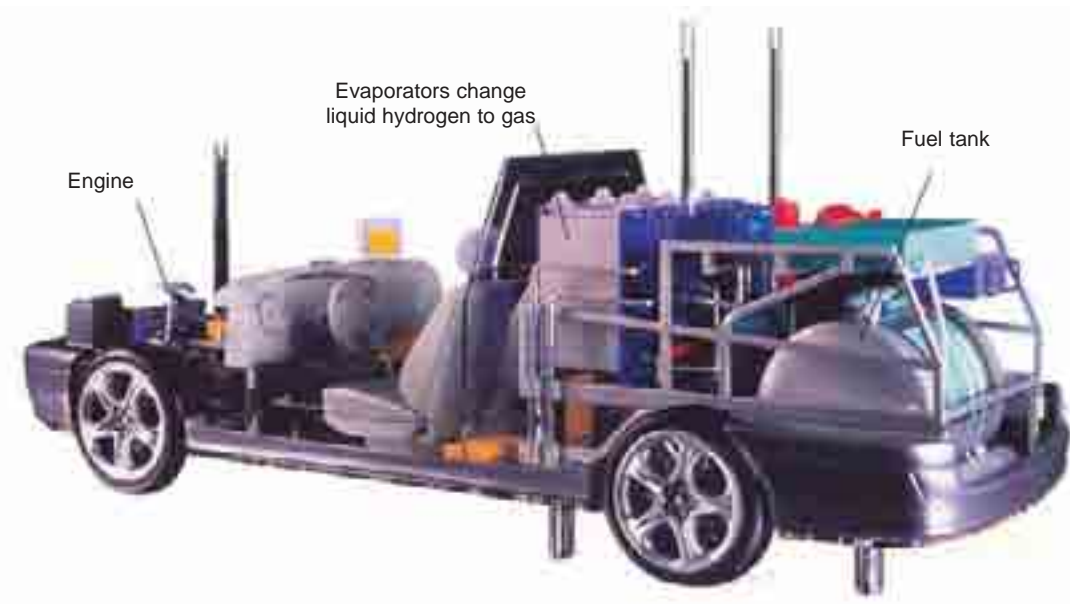
This experimental car burns hydrogen fuel in an ordinary piston engine. Its exhaust gases cause no pollution, because they contain only water vapour.
