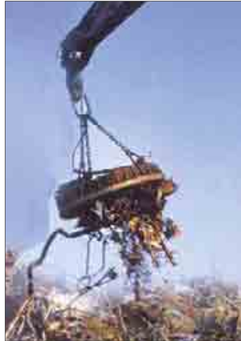
A large disc-shaped electromagnet hangs from jib of this scrapyard crane. Steel and iron objects fly towards the magnet when the current is switched on. In this way, iron and steel can be separated for recycling.
