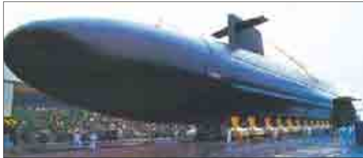
Submarine is akin a to pressure vessel. CAD and CAM were used to design and manufacture this French submarine.
