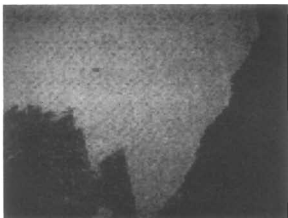
Figure 6 Positive ion image of \text{CF}_3 taken from a 1\text{-mm}^2 area.
